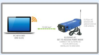
Access Point mode sets the ELITEPRO XC as an access point. View real-time data on a wi-fienabled laptop running ELOG software
