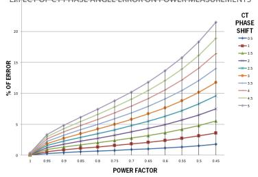
For example, with an uncorrected 3° phase angle error and reported power factor of 0.5, there is a corresponding kW error of >10%.
